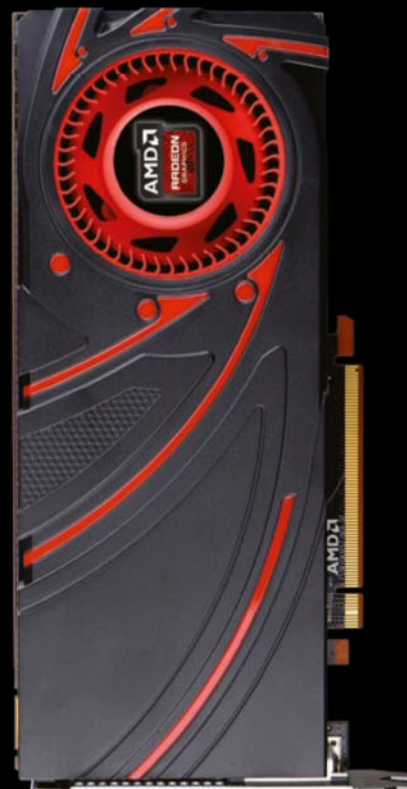
▲ Any GPUs based on AMD's Graphics Core Next architecture, such as the R9 270X, will be compatible with the DX12 spec, but there could still be optional features that require new hardware
